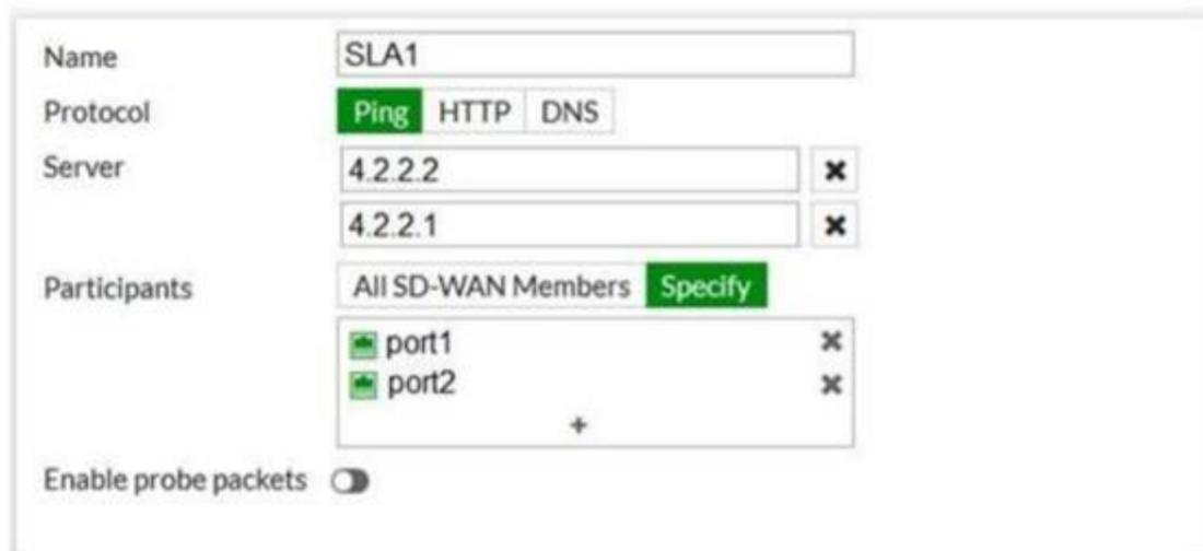
The screenshot shows the configuration for an SLA named 'SLA1'. The 'Protocol' is set to 'Ping'. The 'Server' field contains two entries: '4.2.2' and '4.2.2.1'. The 'Participants' field is set to 'All SD-WAN Members'. There are two ports listed: 'port1' and 'port2'. The 'Enable probe packets' checkbox is unchecked.
