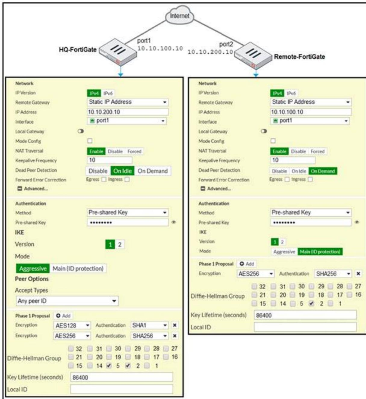
Based on the phase 1 configuration and the diagram shown in the exhibit, which two configuration changes will bring phase 1 up? (Choose two.)
