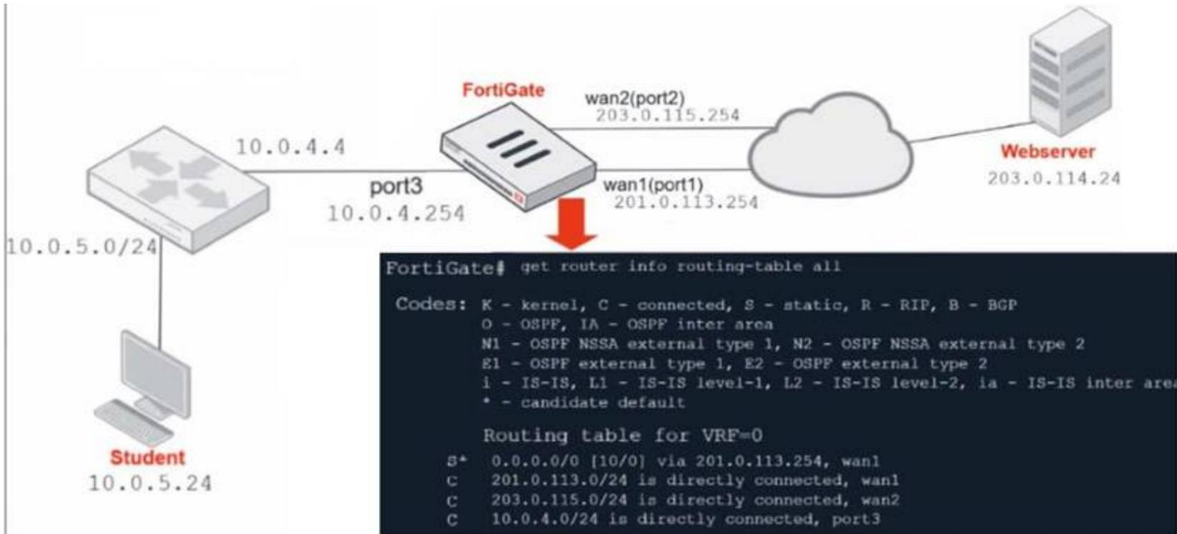
Which contains a network diagram and routing table output. The Student is unable to access Webserver. What is the cause of the problem and what is the solution for the problem?
