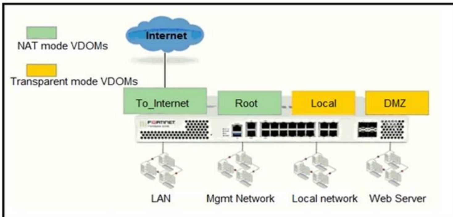
The Root and To\_Internet VDOMs are configured in NAT mode. The DMZ and Local VDOMs are configured in transparent mode. The Root VDOM is the management VDOM. The To\_Internet VDOM allows LAN users to access the internet. The To\_Internet VDOM is the only VDOM with internet access and is directly connected to ISP modem .
