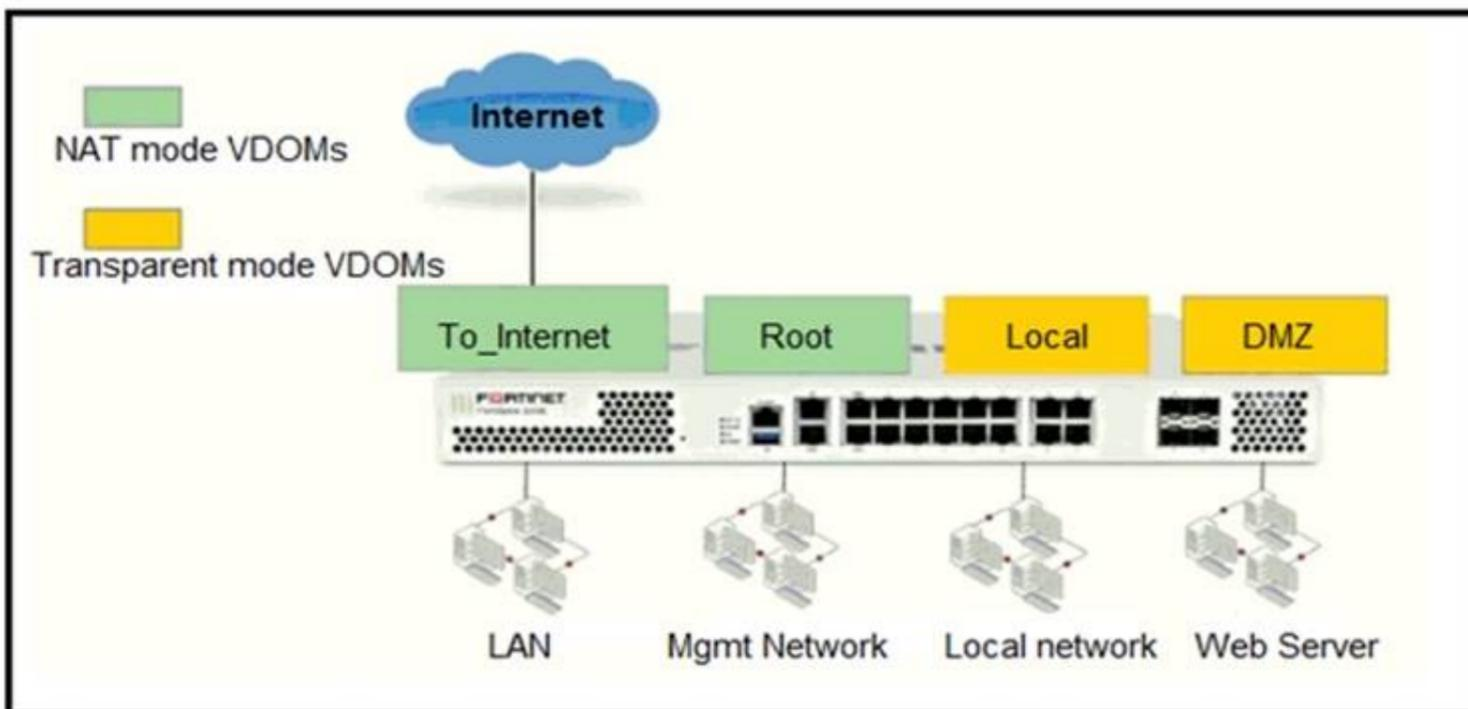
The Root and To\_Internet VDOMs are configured in NAT mode. The DMZ and Local VDOMs are configured in transparent mode. The Root VDOM is the management VDOM. The To\_Internet VDOM allows LAN users to access the internet. The To\_Internet VDOM is the only VDOM with internet access and is directly connected to ISP modem . With this configuration, which statement is true?
