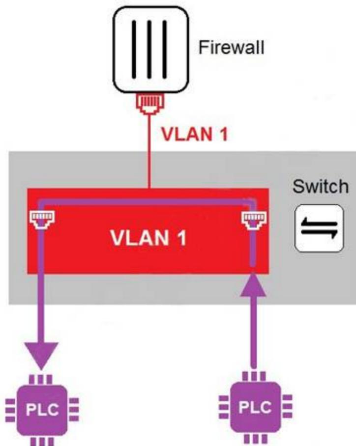
In the topology shown in the exhibit, both PLCs can communicate directly with each other, without going through the firewall. Which statement about the topology is true?
