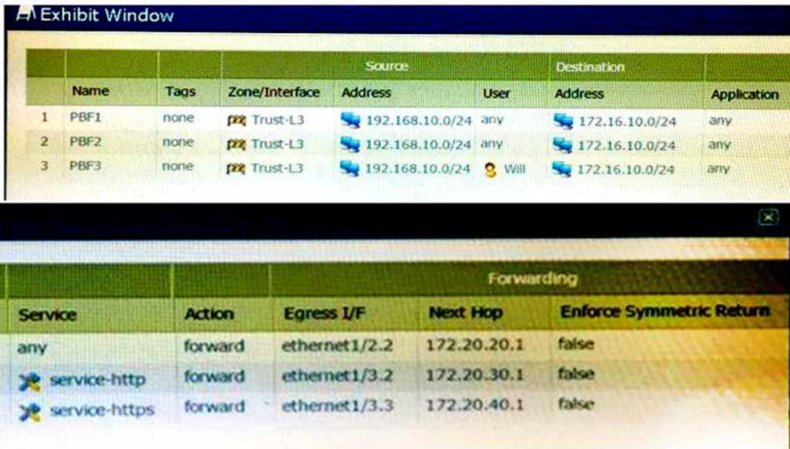
A firewall has three PBF rules and a default route with a next hop of 172.20.10.1 that is configured in the default VR. A user named Will has a PC with a 192.168.10.10 IP address. He makes an HTTPS connection to 172.16.10.20.
