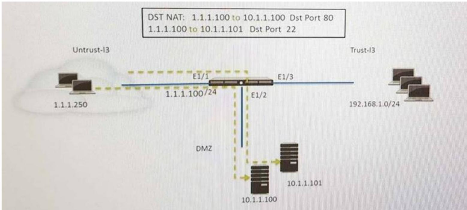
An administrator is using DNAT to map two servers to a single public IP address. Traffic will be steered to the specific server based on the application, where Host A (10.1.1.100) received HTTP traffic and host B(10.1.1.101) receives SSH traffic. Which two security policy rules will accomplish this configuration? (Choose two)
