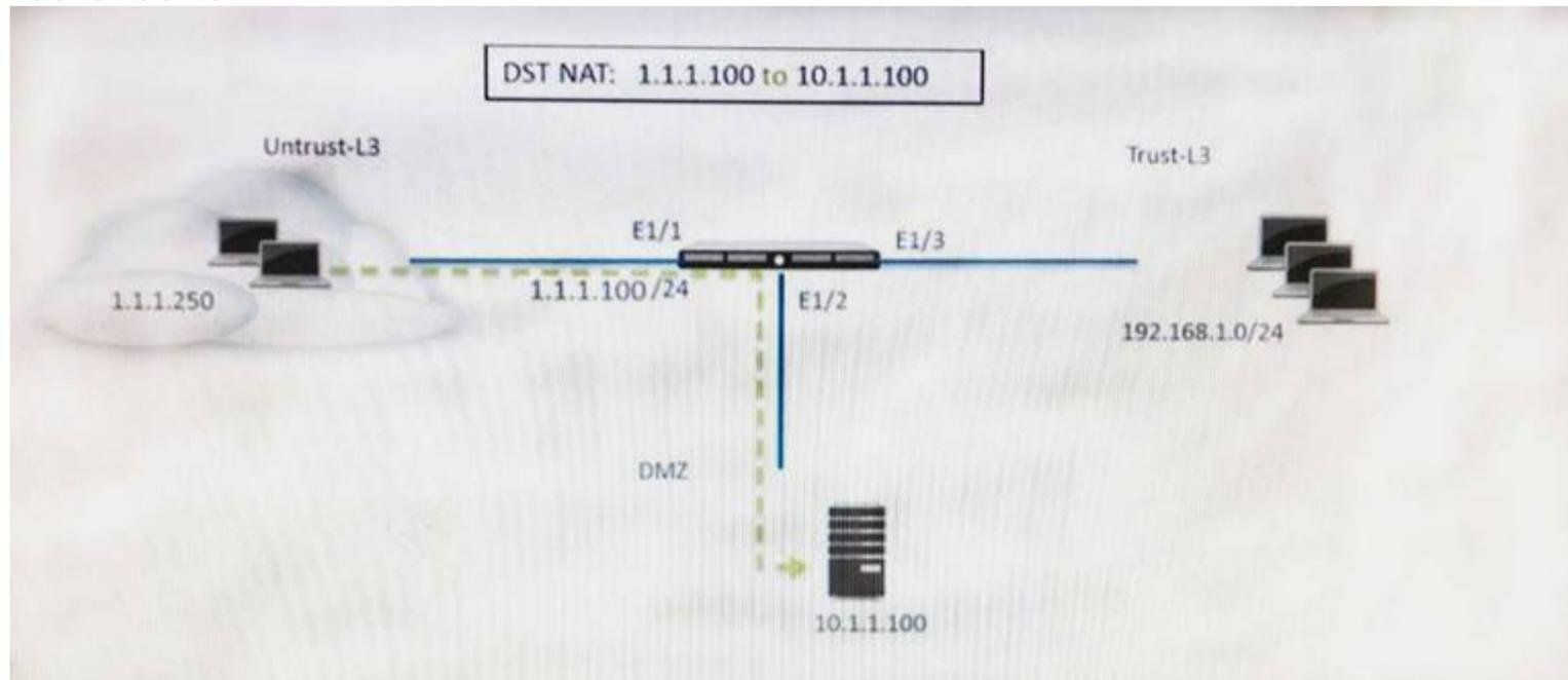
A web server in the DMZ is being mapped to a public address through DNAT. Which Security policy rule will allow traffic to flow to the web server?
