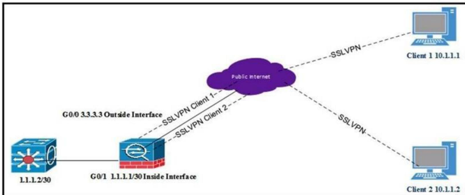
All internal clients behind the ASA are port address translated to the public outside interface that has an IP address of 3.3.3.3. Client 1 and client 2 have established successful SSL VPN connections to the ASA. What must be implemented so that "3.3.3.3" is returned from a browser search on the IP address?
