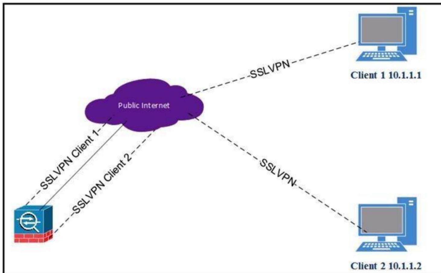
Client 1 cannot communicate with client 2. Both clients are using Cisco AnyConnect and have established a successful SSL VPN connection to the hub ASA. Which command on the ASA is missing?
