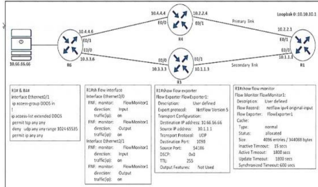
Refer to the exhibit An engineer configured NetFlow but cannot receive the flows from R1 Which two configurations resolve the issue? (Choose two )
