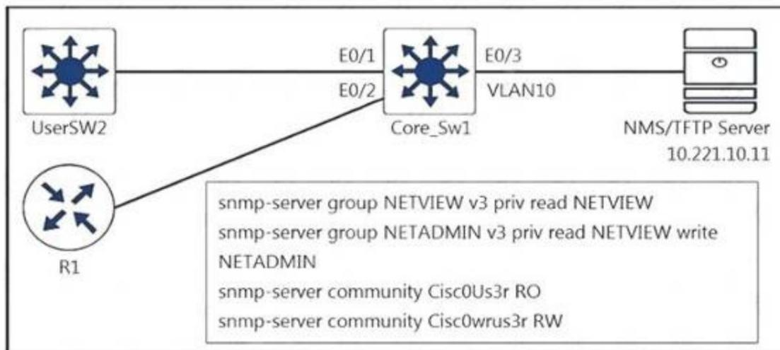
A junior engineer configured SNMP to network devices. Malicious users have uploaded different configurations to the network devices using SNMP and TFTP servers.
