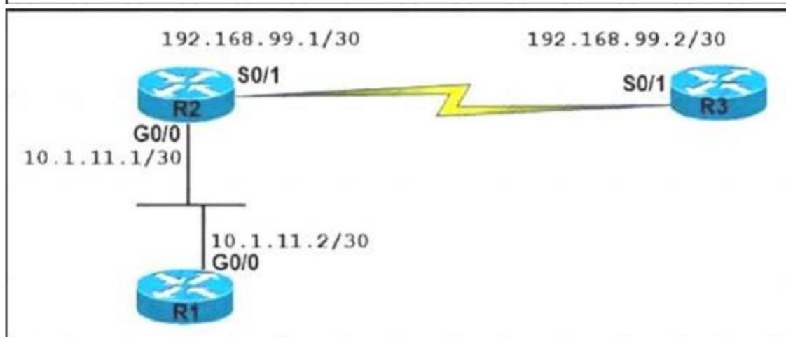
An OSPF neighbor relationship between R2 and R3 is showing stuck in EXCHANGE/EXSTART state. The neighbor is established between R1 and R2. The network engineer can ping from R2 to R3 and vice versa, but the neighbor is still down. Which action resolves the issue?
