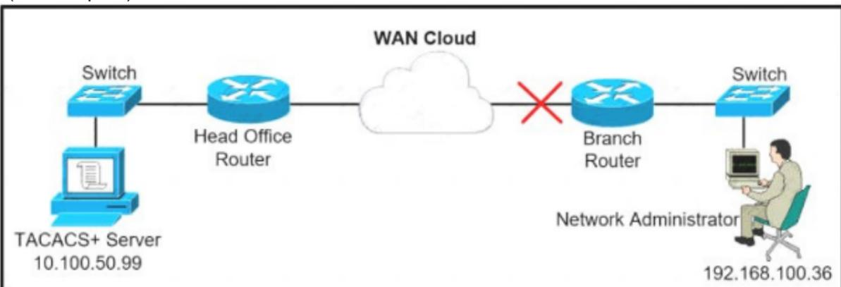
A network administrator is trying to access a branch router using TACACS+ username and password credentials, but the administrator cannot log in to the router because the WAN connectivity is down. The branch router has following AAA configuration:
