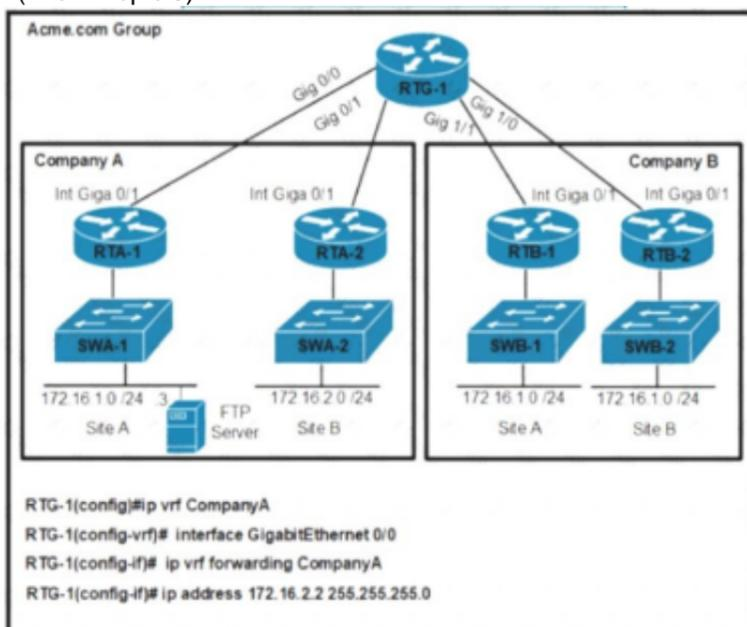
Refer to the exhibit. An engineer must configure a per VRF for TACACS+ for company A. Which configuration on RTG-1 accomplishes the task?
