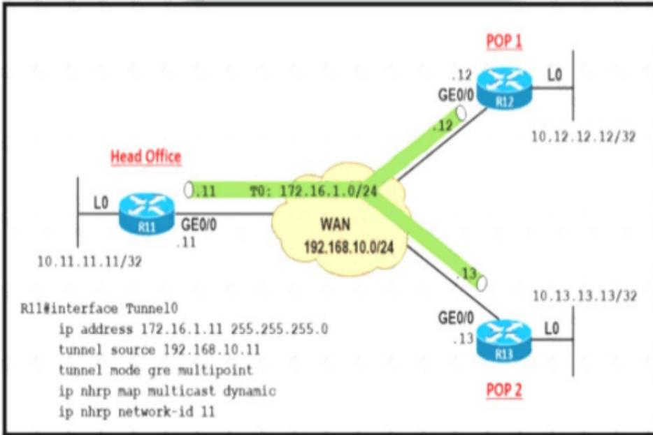
Refer to the exhibit A company builds WAN infrastructure between the head office and POPs using DMVPN hub-and-spoke topology to provide end-to-end communication All POPs must maintain point-to-point connectivity with the head office Which configuration meets the requirement at routers R12 and R13?
