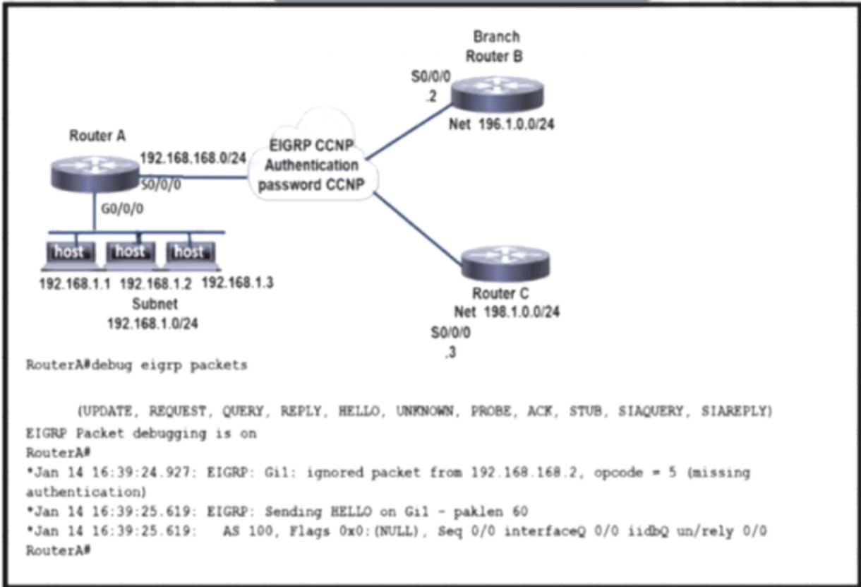
Refer to the exhibit. The services at branch B are down. An engineer notices mal rouser A and router B are not exchanging any routes Which configuration resolves the issue on router B?
