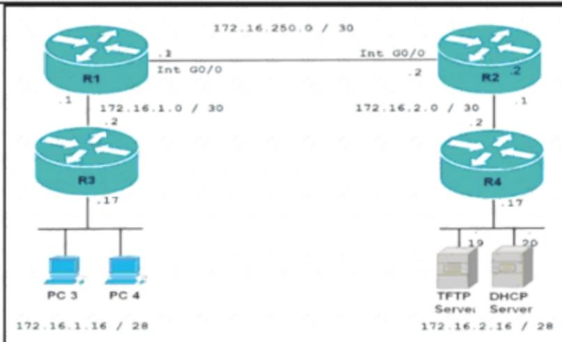
Refer to the exhibit. The engineer is getting an error when trying to transfer a new IOS file to the router. Which action resolves the issue?
