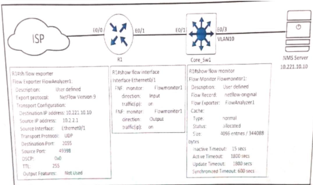
An engineer configured NetFlow on R1, but the NMS server cannot see the flow from ethernet 0/0 of R1. Which configuration resolves the issue?
