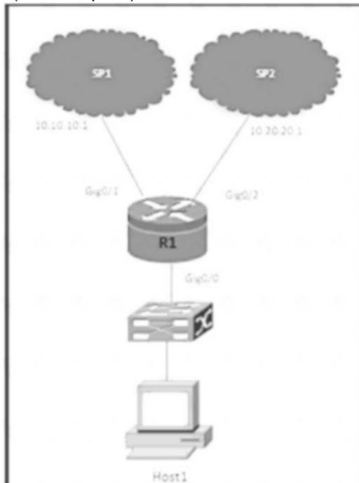
Refer to the exhibit. R1 uses SP1 as the primary path. A network engineer must force all SSH traffic generated from R1 toward SP2. Which configuration accomplishes the task?
