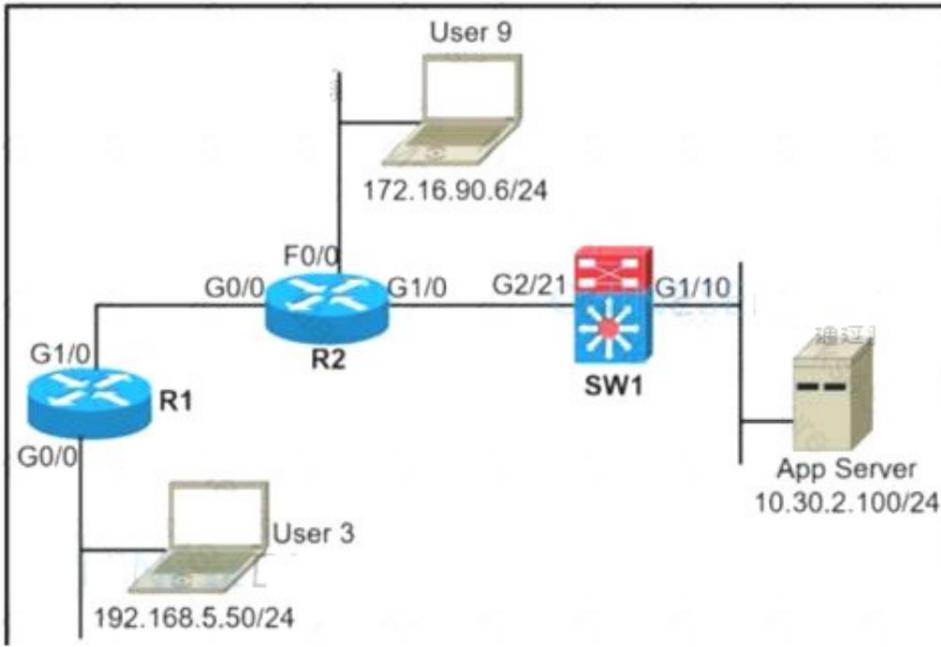
A network administrator must block ping from user 3 to the App Server only. An inbound standard access list is applied to R1 interface G0/0 to block ping. The network administrator was notified that user 3 cannot even ping user 9 anymore. Where must the access list be applied in the outgoing direction to resolve the issue?
