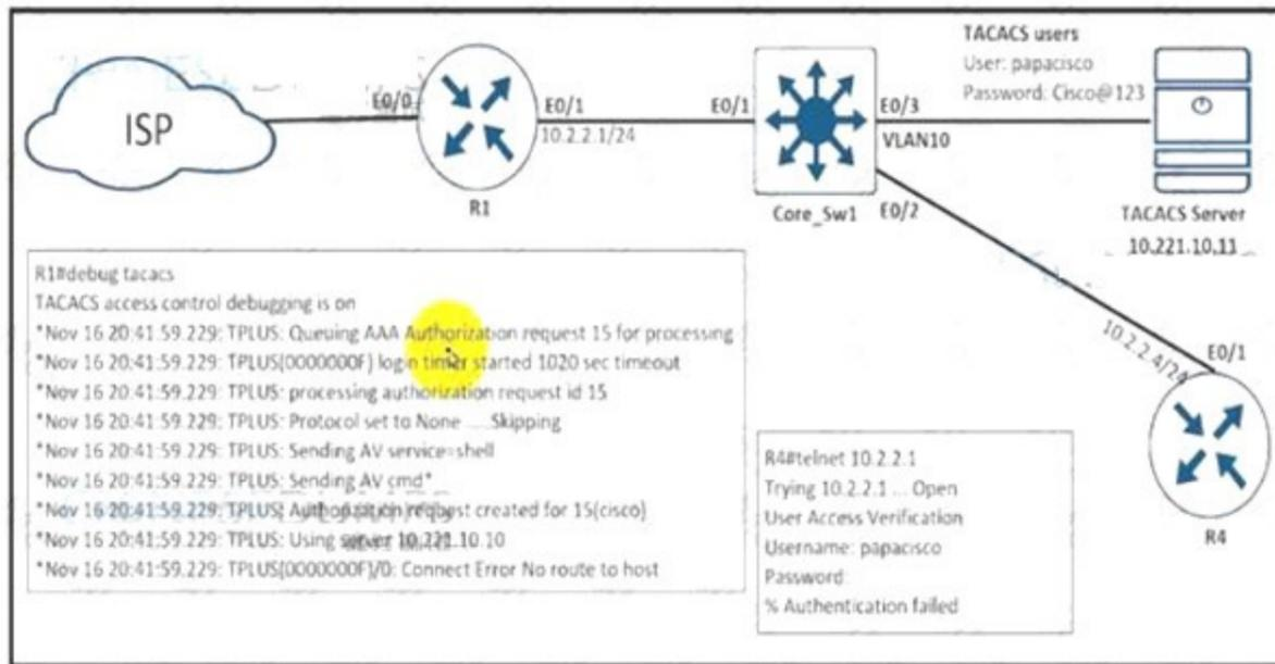
An engineer is trying to connect to R1 via Telnet with no success. Which configuration resolves the issue?
