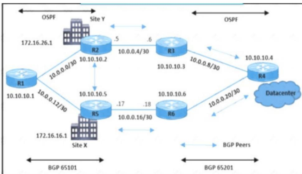
Refer to the exhibit A customer reported a failure and intermittent disconnection between two office buildings site X and site Y The network team finds that site X and site Y are exchanging email application traffic with the data center network Which configuration resolves the issue between site X and site Y?
