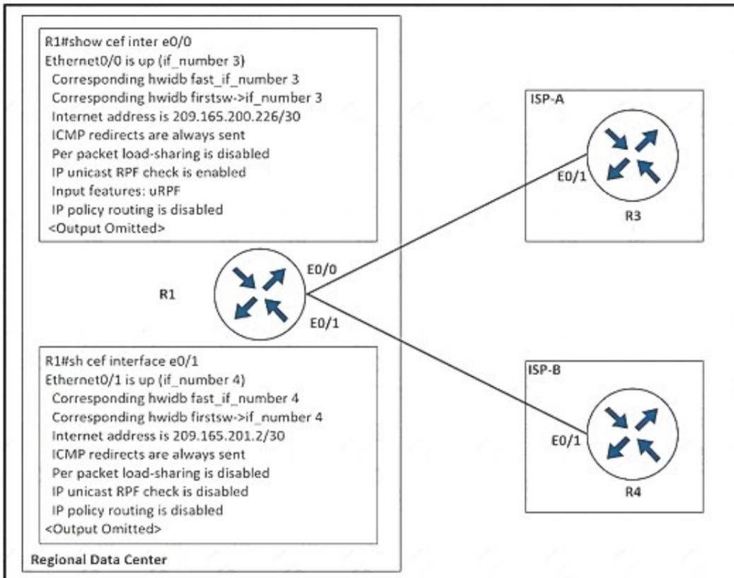
Refer to the exhibit. The company implemented uRPF to address an antispoofing attack. A network engineer received a call from the IT security department that the regional data center is under an IP attack Which configuration must be implemented on R1 to resolve this issue?
