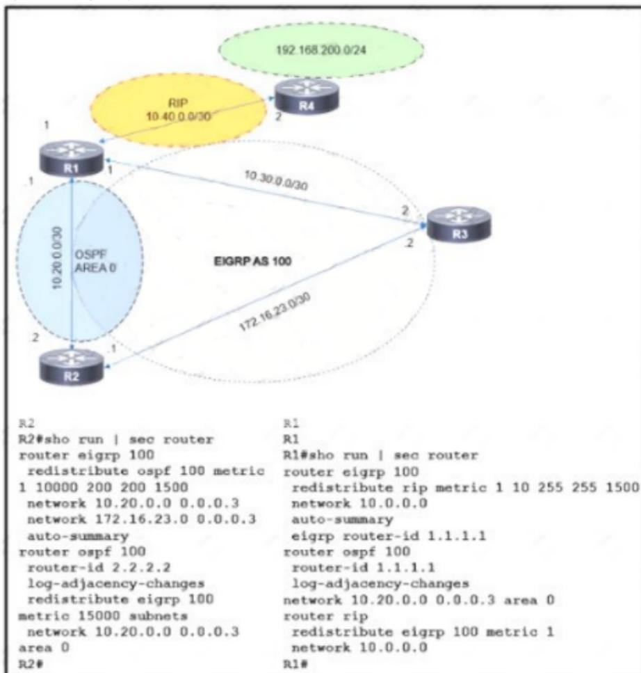
Refer to the exhibit The route to 192 168 200 0 is flapping between R1 and R2 Which set of configuration changes resolves the flapping route?
