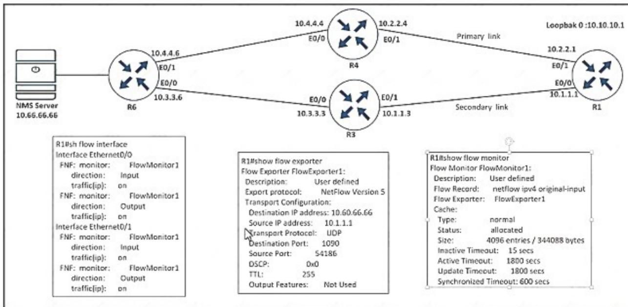
Refer to the exhibit. An engineer configured NetFlow on R1, but the flows do not reach the NMS server from R1. Which configuration resolves this Issue?
