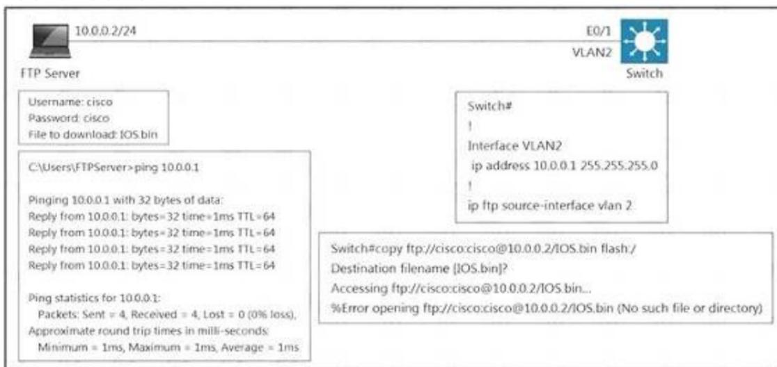
An engineer cannot copy the IOS.bin file from the FTP server to the switch. Which action resolves the issue?
