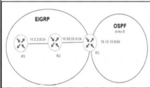
Refer to the exhibit. An engineer configured router R3 to redistribute the prefix 10.10.10.0/24 from OSPF into EIGRP R1 has no connectivity to the prefix. Which action enables receipt of prefixes on R1?
