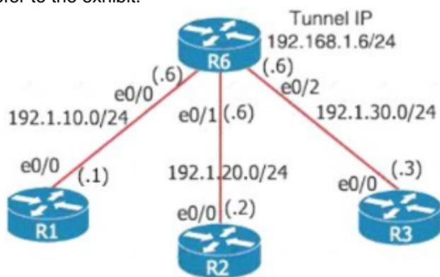
An engineer must establish multipoint GRE tunnels between hub router R6 and branch routers R1, R2, and R3. Which configuration accomplishes this task on R1?
