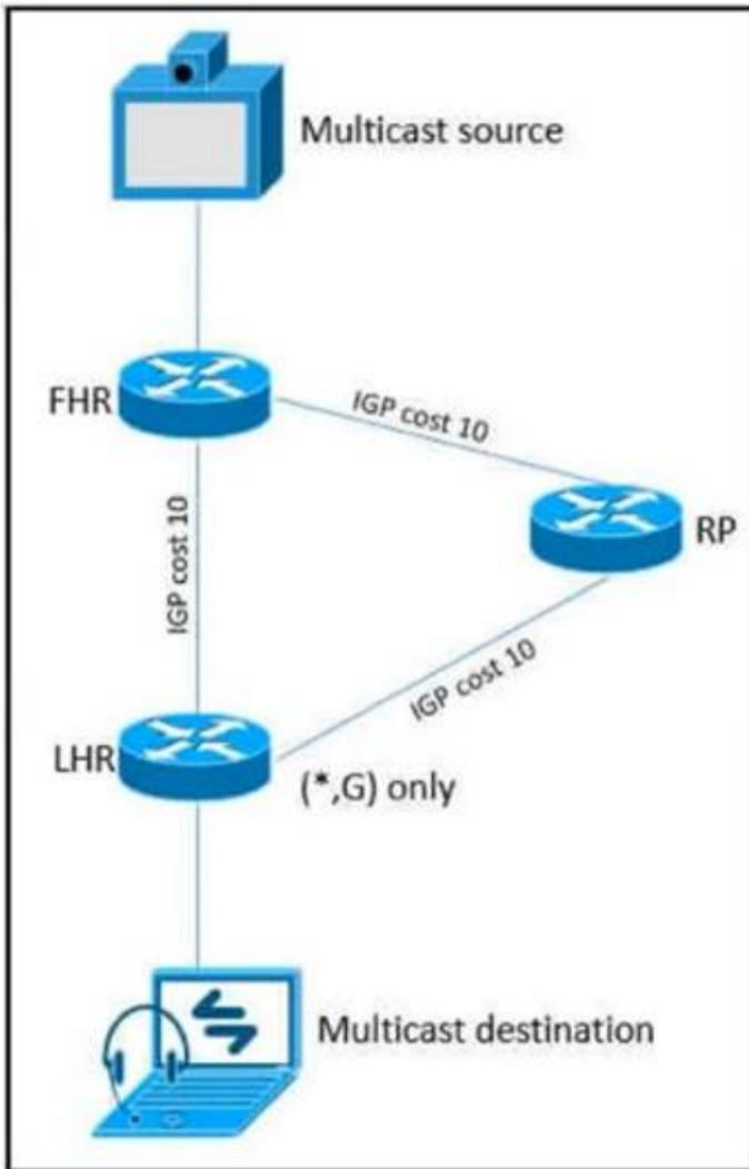
As part of a redesign project, you must predict multicast behavior. What happens to the multicast traffic received on the shared tree (\*,G), if it is received on the LHR interface indicated\*?
