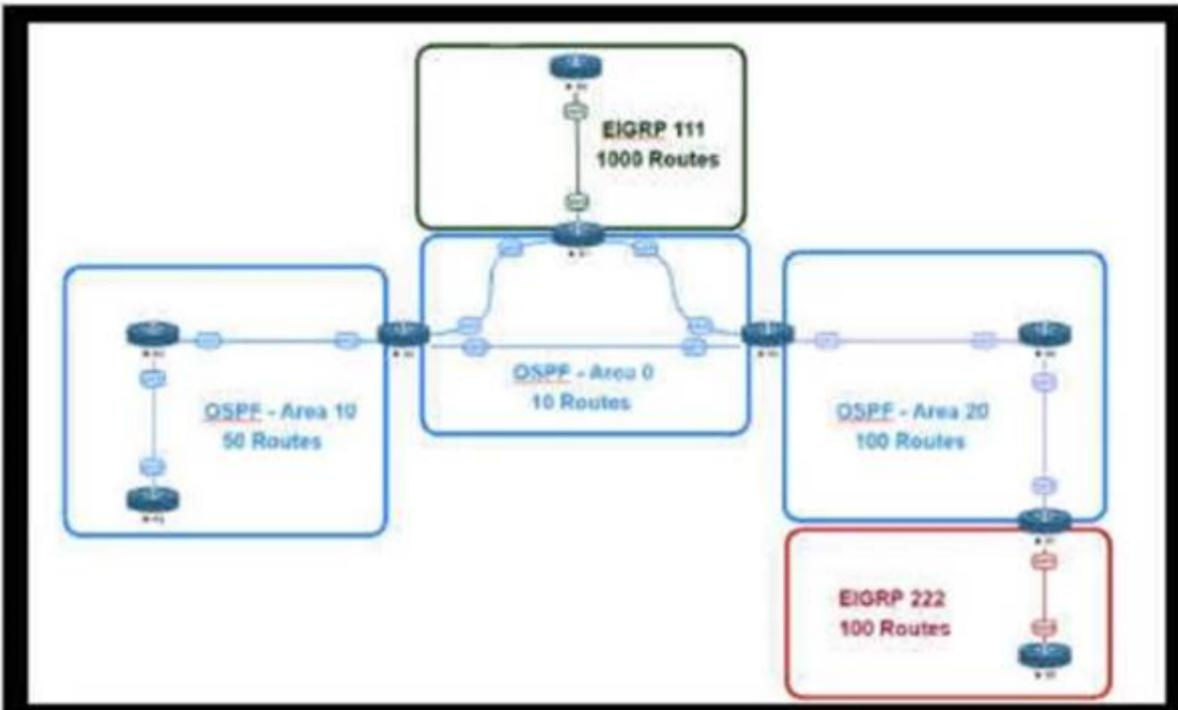
An engineer is designing a multiarea OSPF network for a client who also has a large EIGRP domain. EIGRP routes are getting redistributed into OSPF. OSPF area 20 has routers with limited memory and CPU resources. The engineer wants to block routes from EIGRP 111 from propagating into area 20 and allow EIGRP 222 routes to propagate. In which OSPF area type fulfills this design requirement?
