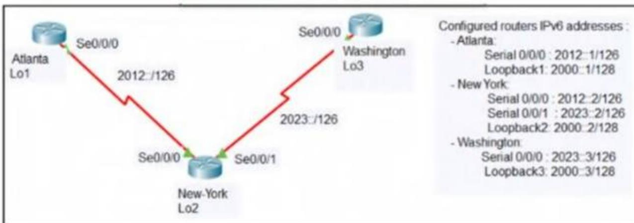
An engineer configured the New York router with state routes that point to the Atlanta and Washington sites. When command must be configured on the Atlanta and Washington routers so that both sites are able to reach the loopback2 interface on the New York router?
