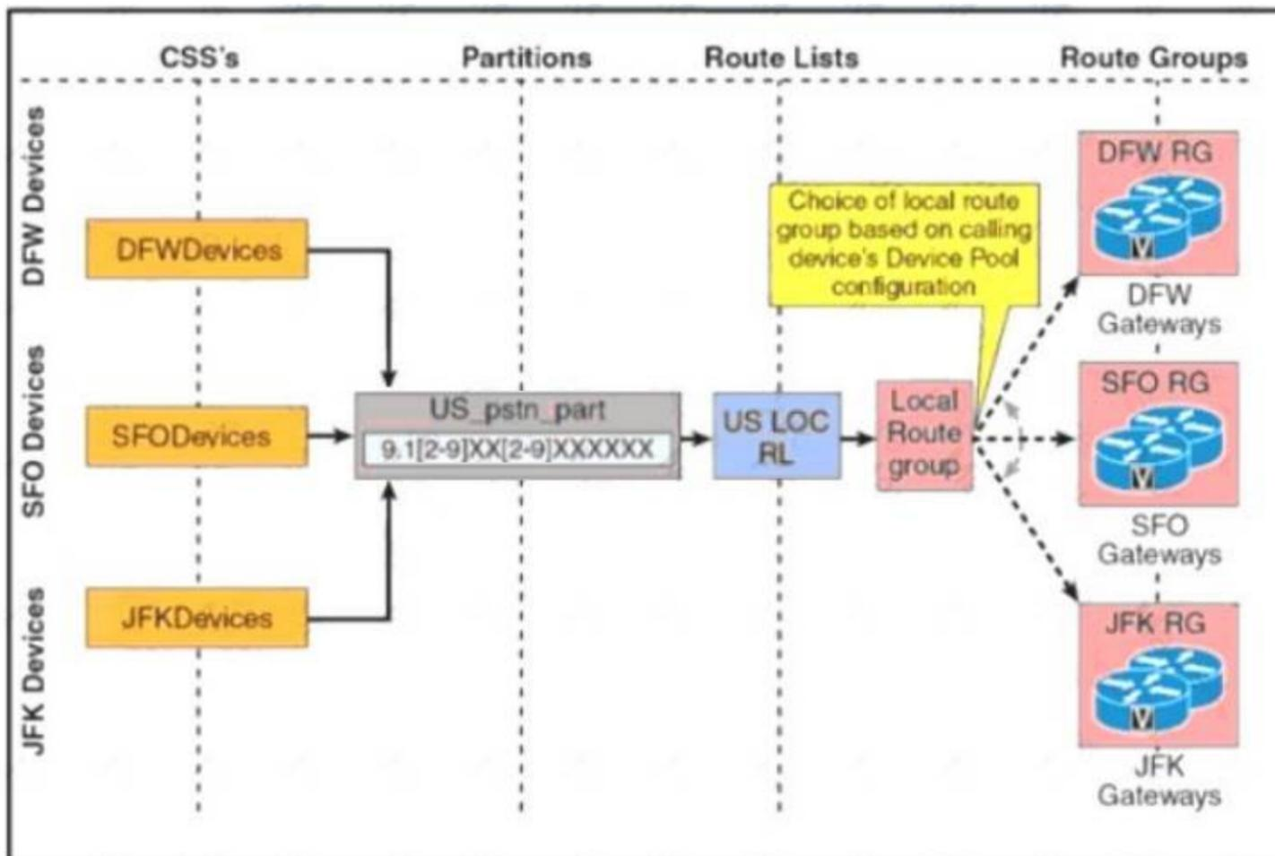
A user takes a phone from San Francisco to New York for a short reassignment. The phone was set up to use the San Francisco device pool, and device mobility is enabled on the Cisco UCM. The user makes a call that matches a route pattern in a route list that contains the Standard Local Route Group. To where does the call retreat?
