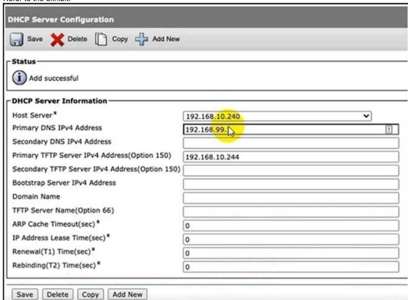
The screenshot shows a web-based configuration interface for a DHCP server. At the top, there is a title bar 'DHCP Server Configuration' with buttons for 'Save', 'Delete', 'Copy', and 'Add New'. Below this is a 'Status' section with an information icon and the text 'Add successful'. The main section is 'DHCP Server Information', which contains several fields:
