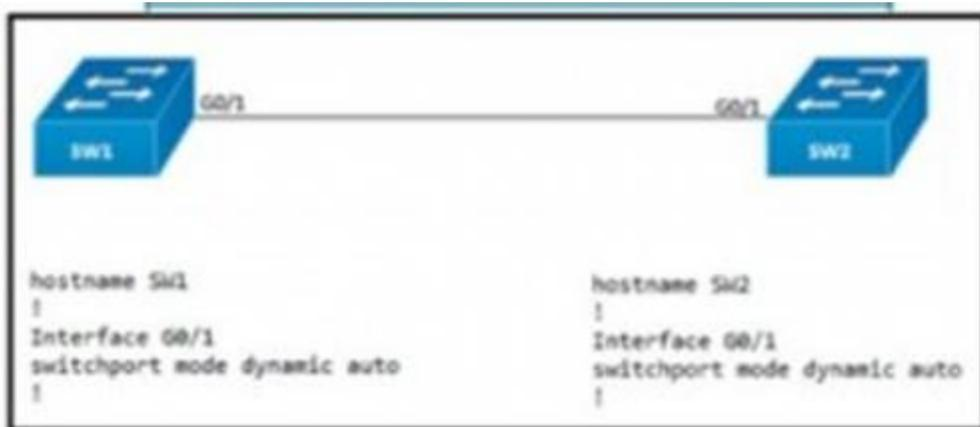
Refer to the exhibit. An engineer attempts to configure a trunk between switch sw1 and switch SW2 using DTP, but the trunk does not form. Which command should the engineer apply to switch SW2 to resolve this issue?
