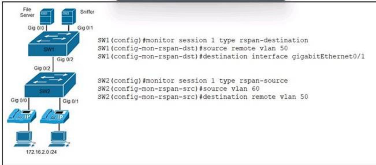
An engineer must send the 172.16.2.0 /24 user traffic to a packet capture tool to troubleshoot an issue. Which action completes the configuration?
