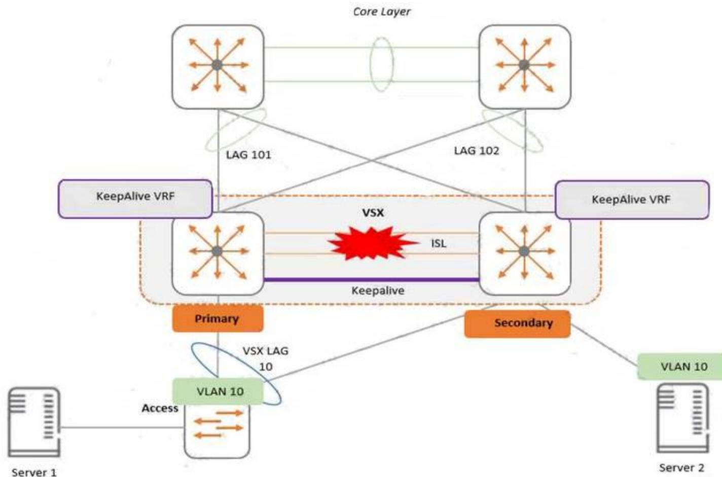
Two AOS-CX switches are configured for VSX at the access layer, where servers attached to them. An SVI interface is configured for VLAN 10 and serves as the default gateway for VLAN 10. The ISL link between the switches fails, but the keepalive interface functions. Active gateway has been configured on the switches. What is correct about access from the servers to the Core?
