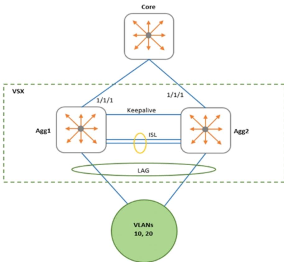
A network administrator is implementing OSPF on a VSX pair of aggregation switches: Agg1 and Agg2. VLANs 10 and 20 are connected to layer-2 access switches. Agg-1 and Agg-2 are configured as the default gateway for VLANs 10 and 20, with active gateway enabled. What is the best practice for configuring OSPF on the aggregation switches and their connection to the Core switch?
