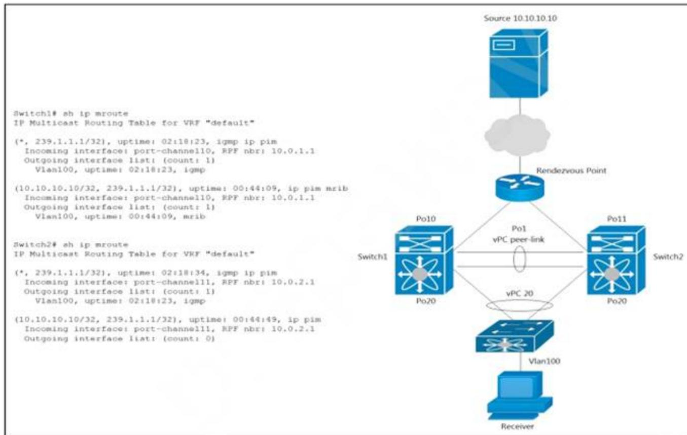
A host with a source address 10.10.10.10 sends traffic to multicast group 239.1.1.1. How do the vPC switches forward the multicast traffic?
