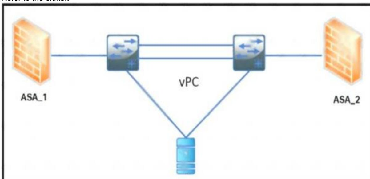
The ASA 1 acts as a Layer 3 gateway for all servers. The servers lose the gateway connectivity when the vPC peer links go down and the vPC keepalive remains up. Which action improves the high availability in the network?
