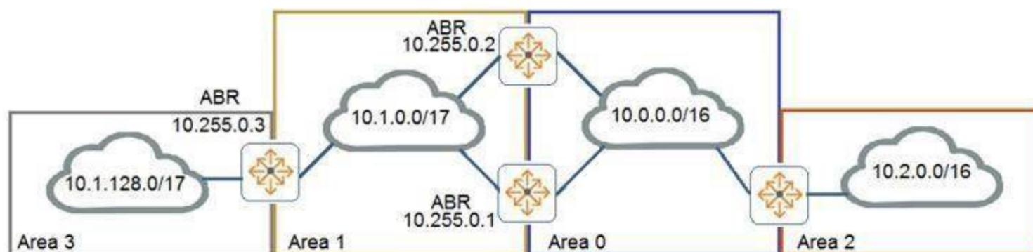
The network administrators is trying to add a remote location as area 3 to the network shown in the diagram. Based on current connection restrictions, the administrator cannot connect area 3 directly to area 0. The network is using AOS-CX switches.
